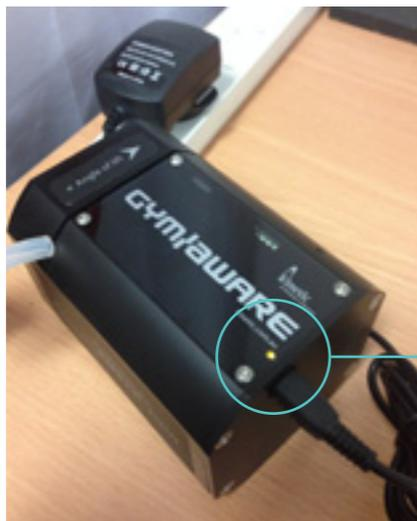
*The PowerTool continuously beeps and the red LED flashes when the tether is not being pulled*
