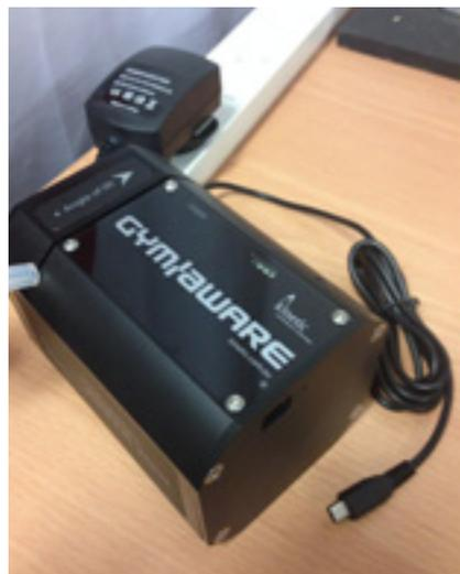
*The red LED starts flashing when the tether is not being pulled.*
