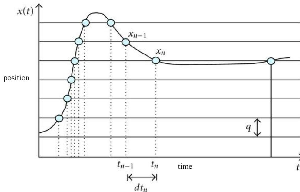
Referring to the figure above, GymAware data points are only recorded when displacement changes by  $q$  (600 microns), when this happens the position is recorded and timestamped ( $dt_n$  in the figure) with a resolution of 35 microseconds - that's equivalent to a sampling rate of 29kHz!
