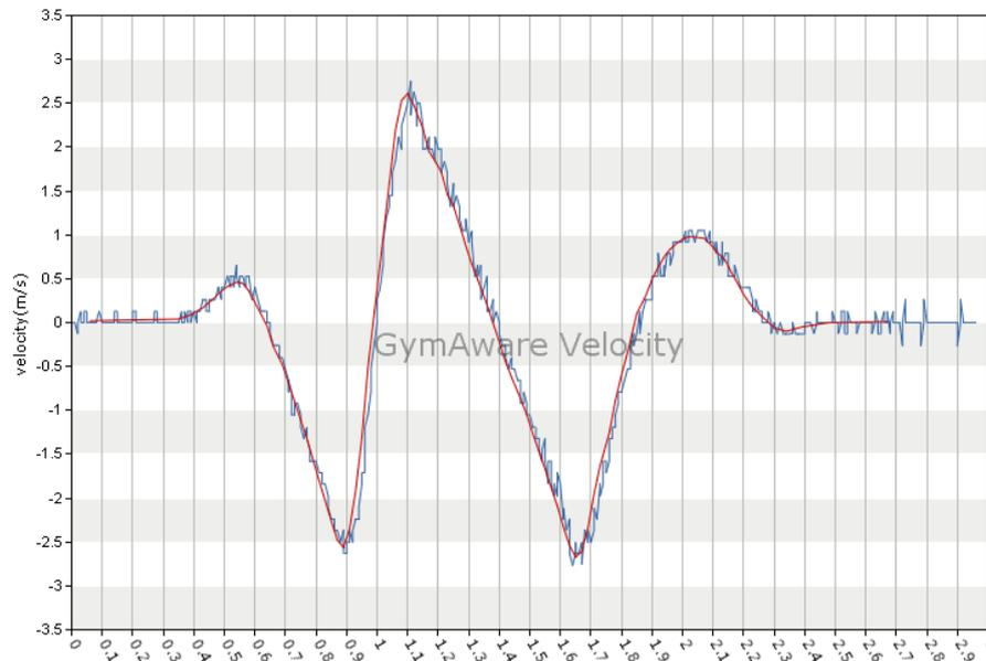
Above is an overlay of raw velocity from a jump recorded simultaneously with GymAware (Red) and the BMS system that uses the traditional 200Hz approach (Blue). Note the amplification of noise due to differentiation. Now lets look at the same signal differentiated again for acceleration:
